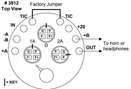
Note: This circuit is designed to use the type 200 & 201 tubes with 5 volt 1 amp filaments.
