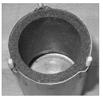
Antenna can with ferrite shield.
