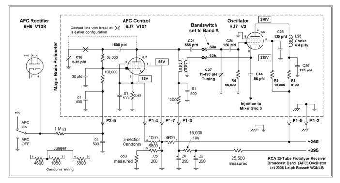
Broadcast band (AFC) oscillator schematic. Components outside the Magic Brain perimeter were measured and may not reflect the exact circuitry in the set.
