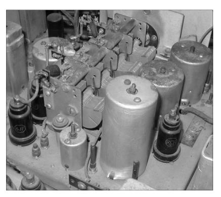
The Magic Brain section of the radio is shown here. Note the fourgang tuning capacitor.
