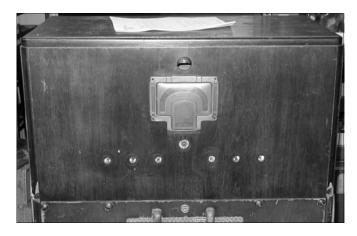
The cabinet of the prototype. The receiver portion is crudely made out of plywood, and sits atop a standard RCA speaker cabinet.
