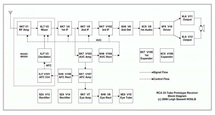
Block diagram of the prototype receiver.
